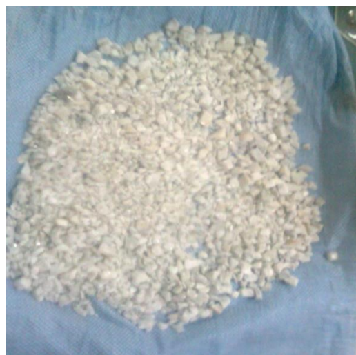
Fig Broken marbles after pulverization(size less than 10mm)
