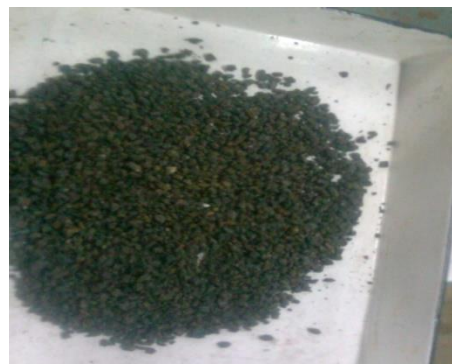
Fig Steel slag after broken less than 10mm
