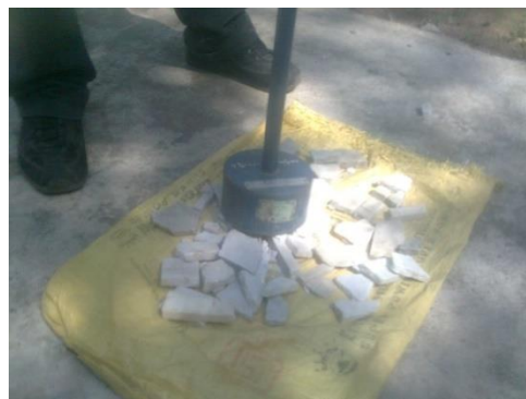
Fig Process of pulverizing the construction waste marbles
