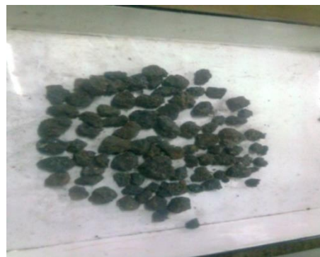
Fig Steel slag before broken less than 10mm
