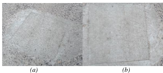
Fig. 12. CFC overlay (a) without hair fibre; (b) with hair fibre
