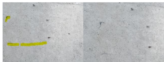
Fig. 15. CFC overlay with hair fibre
