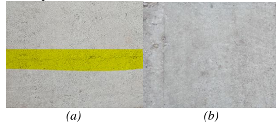
Fig. 13. WTC overlay (a) without hair fibre; (b) with hair fibre
