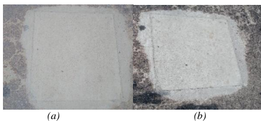
Fig. 11. WTC overlay (a) without hair fibre; (b) with hair fibre
