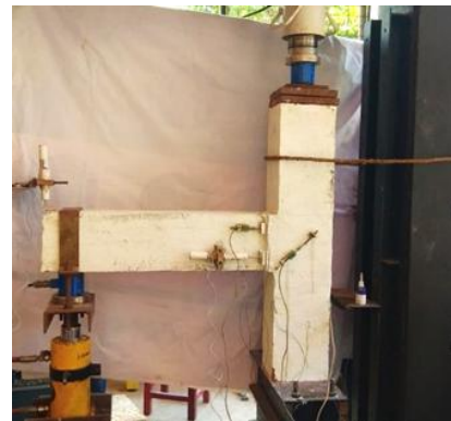
Fig. 4 Test setup of beam-column joints
