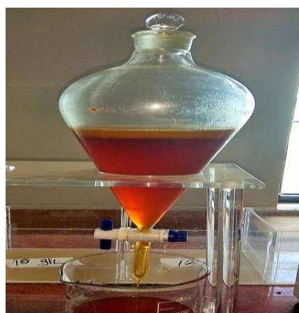
Fig. 2 Transesterified product in separating funnel
