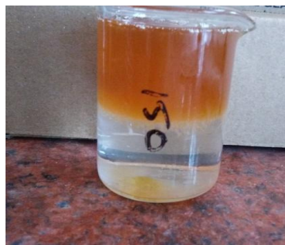
Fig. 3 Transesterified product backwashed with distilled water
