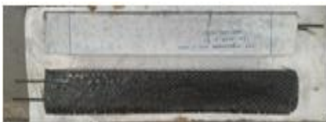
Fig. 7 Specimens strengthened with CFRP sheets
