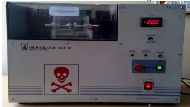
Figure 1: Set up used for Measurement of Breakdown Voltage at Room Temperature
