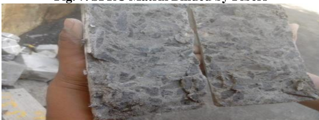
Fig. 8. Control Specimen Splits in Exactly Two Parts
