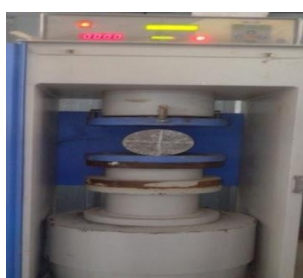
Fig.5. Split tensile Strength Testing of Cylinder.
