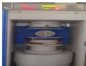
Fig.5. Split tensile Strength Testing of Cylinder.
