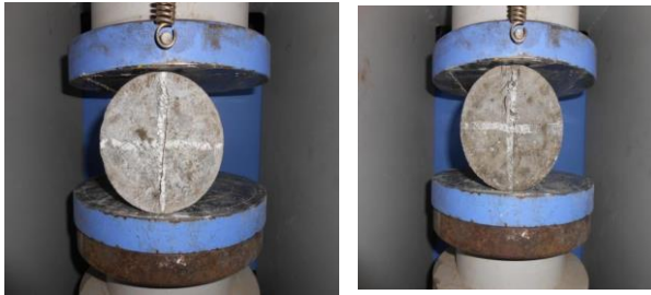
Fig.6. Crack formation in cylinder. (a) Control specimen (b) Specimen with FRC.
