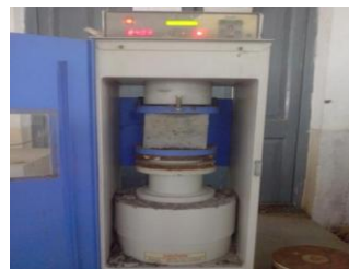
Fig.4. Compressive strength test of Cube.
