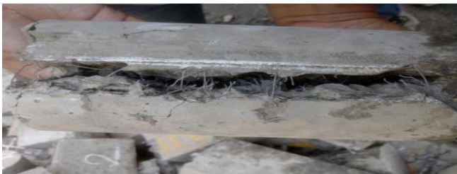
Fig. 7. SFRC Matrix Binded by Fibers
