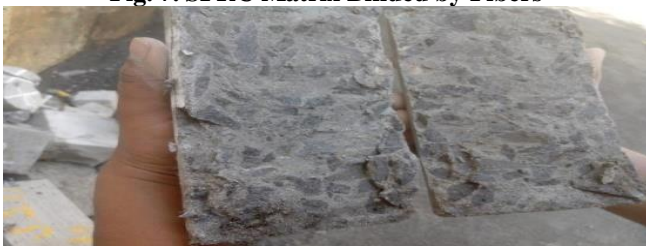
Fig. 8. Control Specimen Splits in Exactly Two Parts
