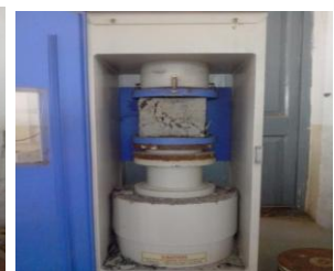
Fig.5. Failure of Cube
