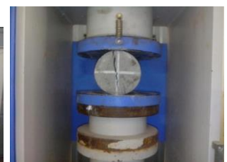
Fig.5. Split tensile Strength Testing of Cylinder.
