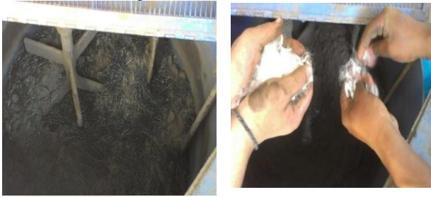
Fig.1 Mixing of fibers- (a)Steel fibers (b) Polypropylene fibers.
