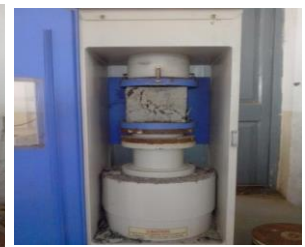
Fig.5. Failure of Cube test of Cube.
