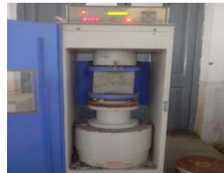
Fig.4. Compressive strength test of Cube.
