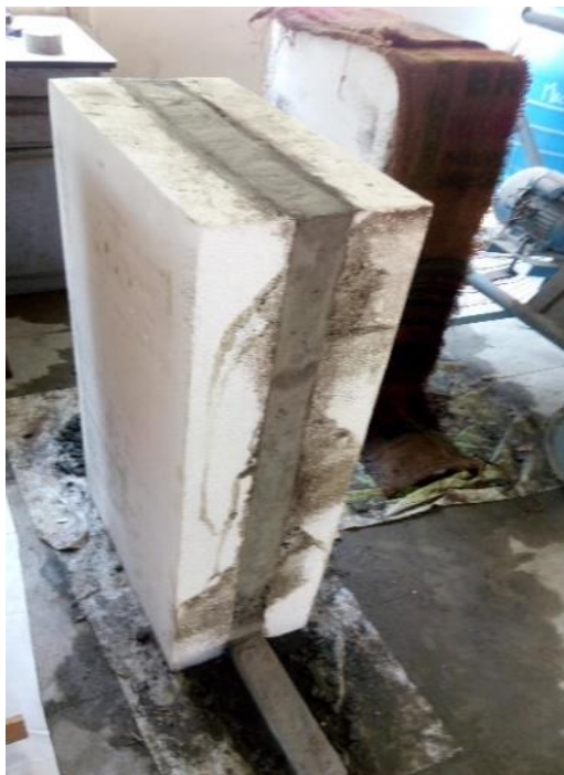
Fig 1. Typical Cast ICF wall Panel
