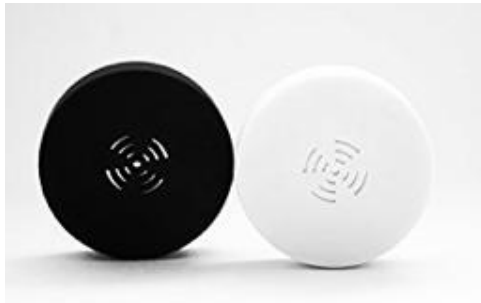
Fig. 4. i Beacon Device powered by Bluetooth Low Energy 4.1.
