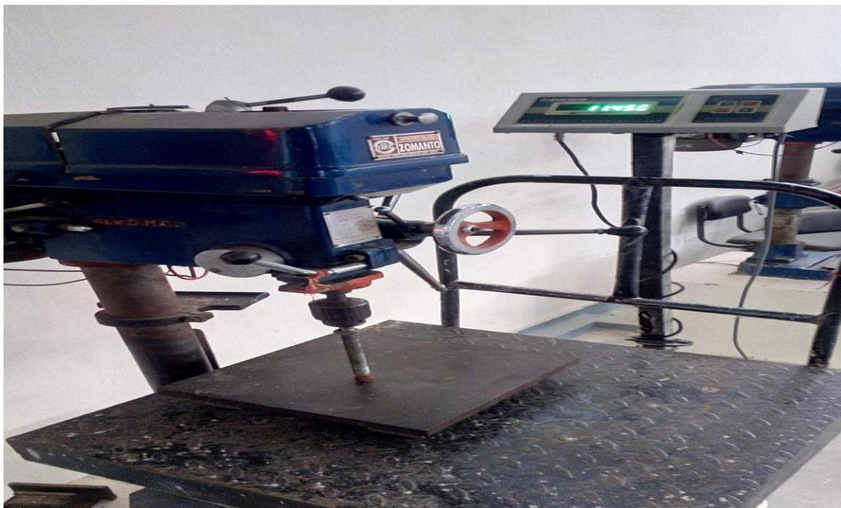
Fig. 2. Machine to Measure the Compressive Strength of Rudraksha Bead
