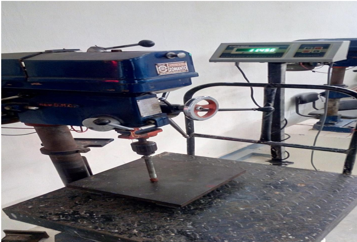
Fig. 2. Machine to Measure the Compressive Strength of Rudraksha Bead
