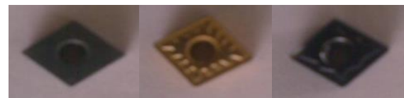
Figure 3. Photographic images of (i) Tungsten carbide Uncoated Tool (ii) Tungsten carbide Tool coated with Titanium Nitrate (iii) Tungsten carbide Tool coated with Aluminum Oxide
