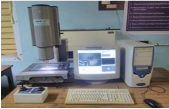
Figure 4. Measurement of Tool wear using Rapid I
