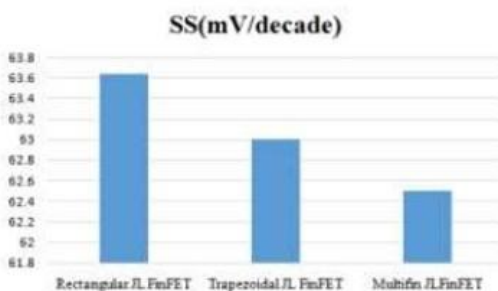
Fig. 13. Comparison on Subthreshold Slope
