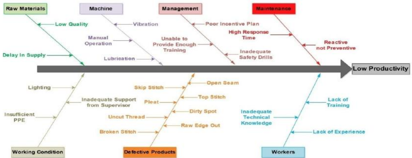
Fig: 4.5 Cause and Effect Diagram for Low Productivity in the Garments Factory.
