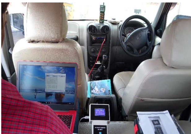
Fig. 3 IAQ Monitor with DAQ
