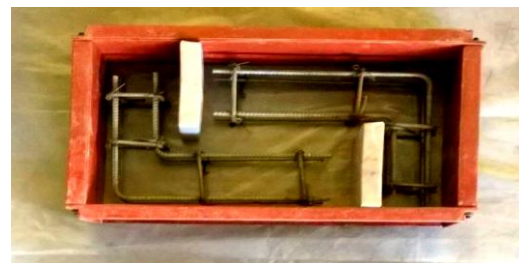
Figure 3. Push-Off Specimen with Reinforcement
