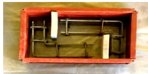
Figure 3. Push-Off Specimen with Reinforcement
