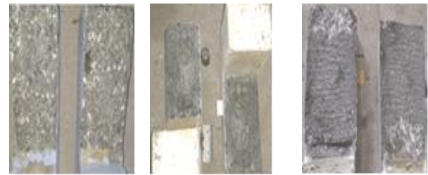
CSM SSM SRM Figure 12. Failure Modes of Interfaced Specimen
