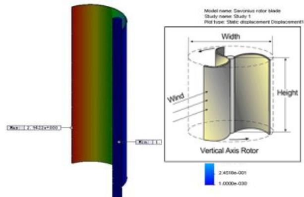
Material used for Blade is E Glass Fiber [4,5]. According to analysis it is seen that at 5m/s wind speed maximum deformation of the blade is 2.9422mm. This shows the design is safe.
