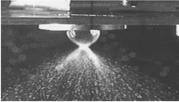
Figure-1 Fuel Spray Pattern of Mark1
