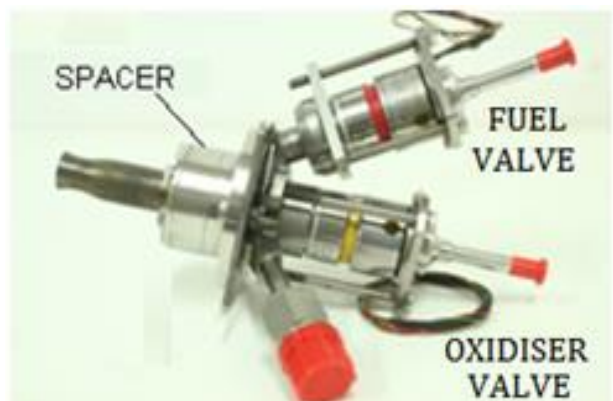
Figure-3 Thruster assembly with Mark1 and type1 (with 11.16 \times 10^{-3}m thick spacer) chamber
