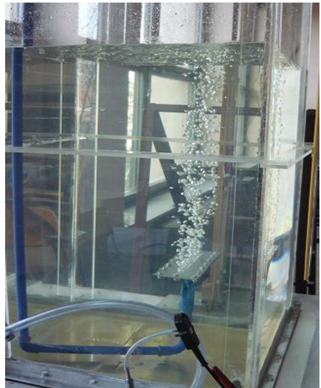
Fig. 5 Working FBG; \Delta h_1 = 60 \text{ mbar} = 611 \text{ mm H}_2\text{O} , Fig. 6 Bubble columns that generate a planar jet; picture made from a lateral side for the figure 5.
