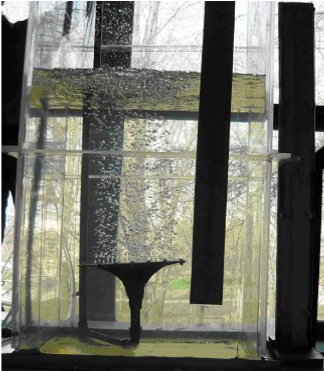
Fig. 5 Working FBG; \Delta h_1 = 60 \text{ mbar} = 611 \text{ mm H}_2\text{O} , Fig. 6 Bubble columns that generate a planar jet; picture made from a lateral side for the figure 5.
