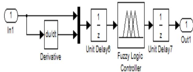
**Fig 13.fuzzy logic controller in simulation**
