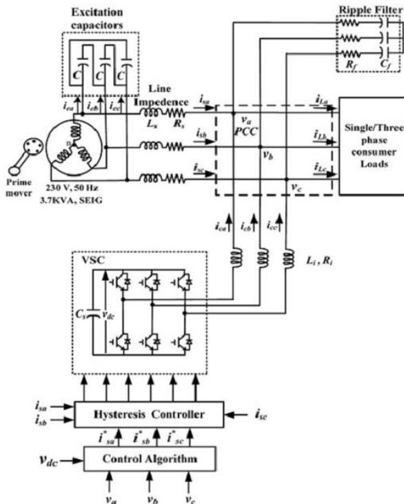
**Fig. 1a. Configuration of DSTATCOM supported induction generator a Schematic diagram of induction generator supported by VSC-based DSTATCOM**
