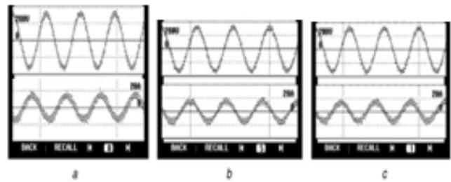
Fig. 11 Performance of DSTATCOM under linear load a Waveforms of vsa and isa b PL and QL c PS and QS
