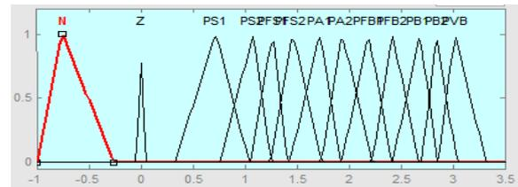
**Fig.9 output variable Membership functions**
