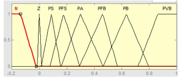
**Fig 7 input error as membership functions**
