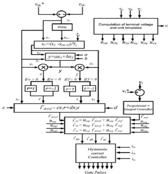
**Fig. 1b. Configuration of DSTATCOM supported induction generator Control algorithm of DSTATCOM for estimation of reference currents using SMC with fuzzy controller**
