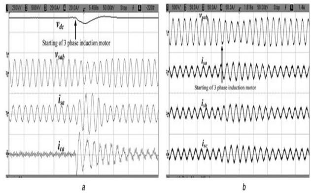
**Fig. 6 Dynamic response of DSTATCOM under induction motor starting along with non-linear loads a, b Variation of parameters such as  $v_{dc}$ ,  $v_{sab}$ ,  $i_{sa}$ ,  $i_{sb}$ ,  $i_{sc}$ , and  $i_{ca}$  during starting of one horse power three-phase induction motor**
