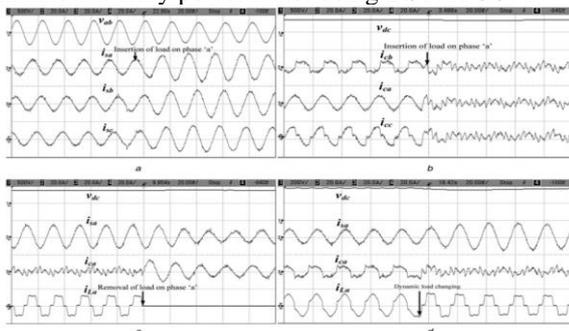
Fig. 10 Dynamic response of DSTATCOM a Removal of load on phase ‘a’ b, c Insertion of load on phase ‘a’ d Sudden load change
