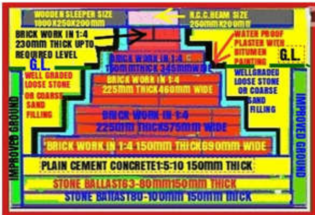
Figure4-Designed/Developed Foundation for Earthquake & Flood Prone Areas
