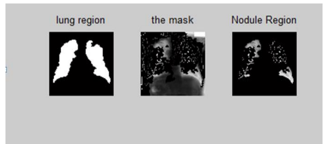
Figure 8: Applying the mask (The lung region and the mask are element by element multiplied to get the nodule region) Thus the final output image is as shown
