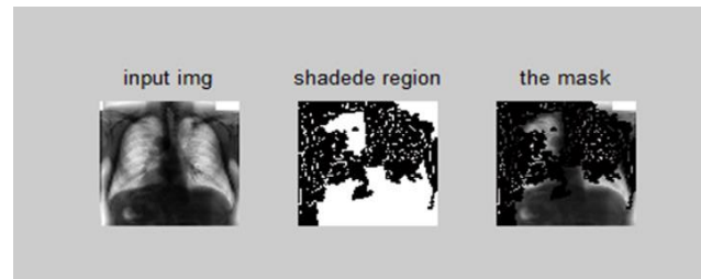
Figure 7: Obtaining the mask (The input image and the shaded watershed image are element by element multiplied to get the mask)
