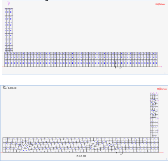
Fig.3 Initial numerical wear model a) initial geometry and mesh b) after global remeshing.
