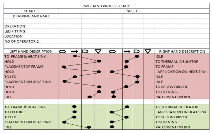
Table VII: Operation: Assembly of Leaf Frame and Heat Sink
