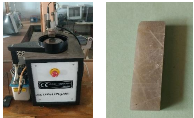
Figure 13 : Wear Test Figure 14: Wear Test Sample Machine
