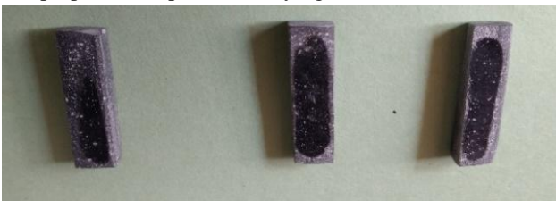
Figure 2 : Raw Samples of Epoxy Resin with Filler Materials
