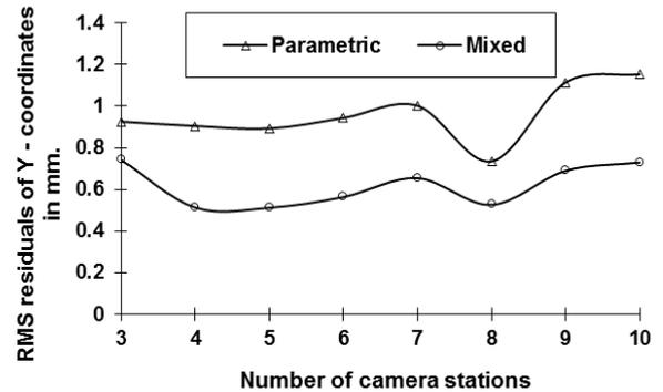
Figure(4): The relation between RMS residual of Y-coordinates the number of Camera Stations
