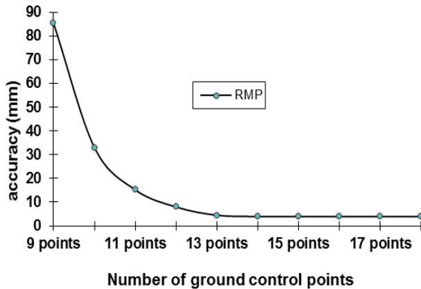
Figure (2): The relation between the accuracy and the number of ground control points obtained from the parametric adjustment technique
