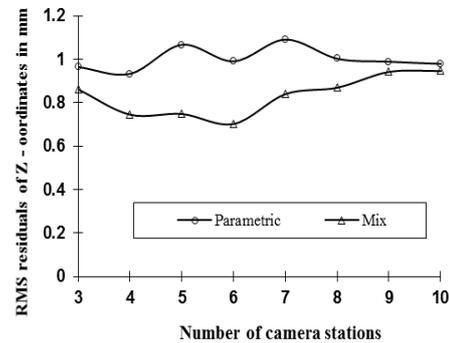
Figure(5): The relation between the RMS residual of Z-coordinates the number of camera
