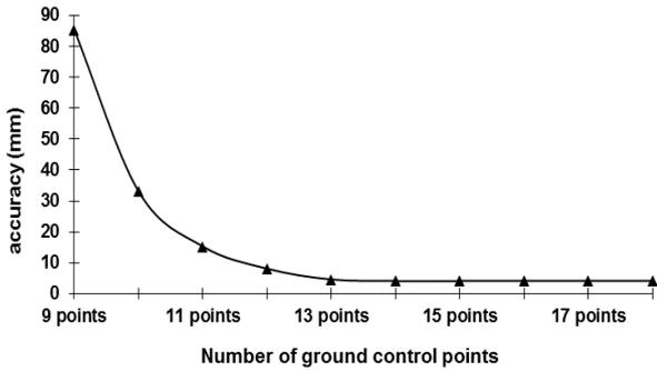
Figure (1): The relation between the accuracy and the number of ground control points obtained from the mixed adjustment technique
