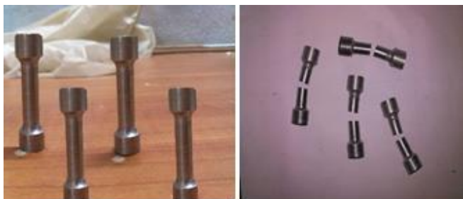
Fig 3: Specimen before Test & After Test Using Electronic Tens Meter
