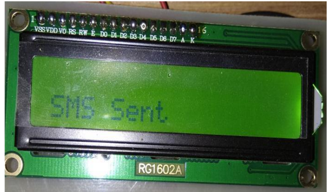
Pic-6. After the Fault Occurred The System Sent SMS To Authorized Person.
