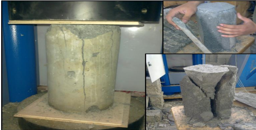
Figure 5: Mode of failure of UHPC cylinder.
