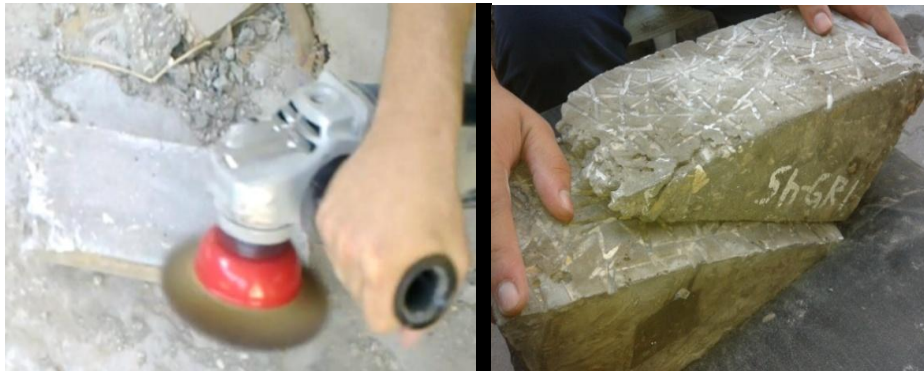
Figure 3: Wire brush and Random Scarifying Treatment Techniques.
