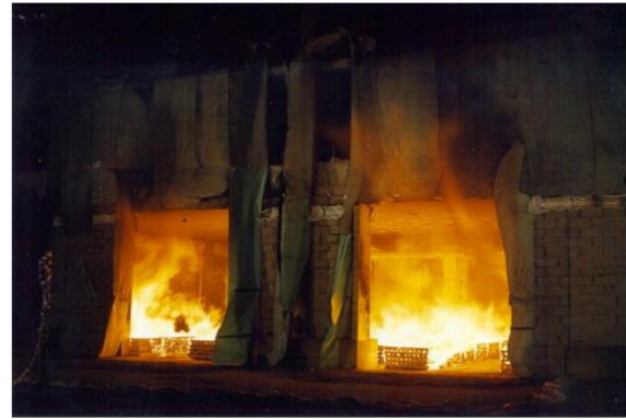
Fig.6. Full scale Cardington Fire test
