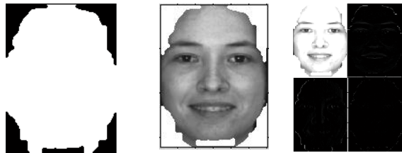
a)Mask image of Enhanced CLAHE image b) Gray-scale image using mask c)DWT's four sub images L1, H1, V1 and D1
