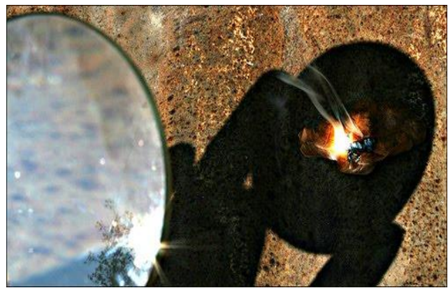
Fig. 4. Using spherical mirrors and Fresnel lenses to melt plastic.
