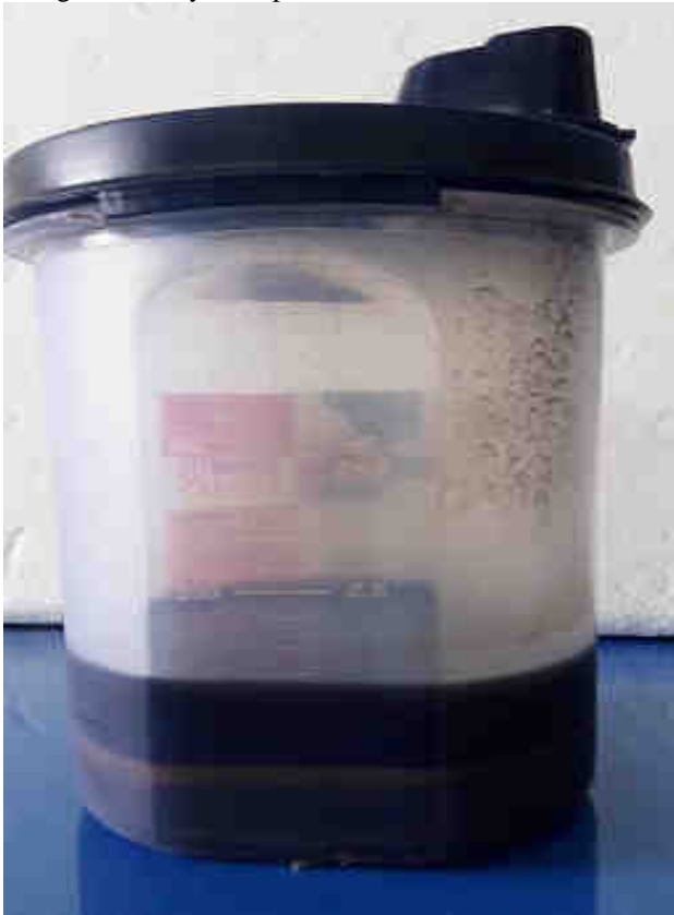
Fig. 2. Gravitational settling of iron particles
