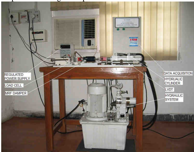
Fig:5. Experimental setup of MRF damper
