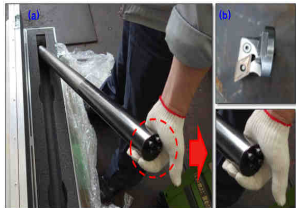
Fig. 1 Installed non-vibration bars (dampened bars)
