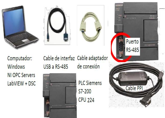
Fig 5. Equipment and cables used in communication with MATLAB® or LabVIEW®.
