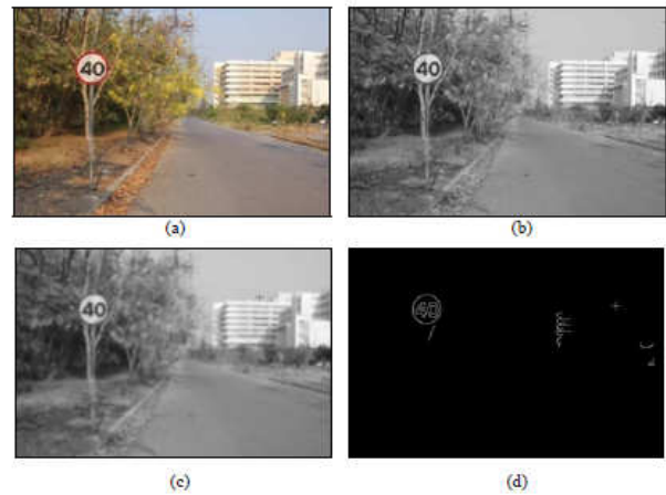
Fig 3 : (a) Color Mode Image,(b) Black and White Mode Image,(c) Smooth Image, (d ) Binary Image
