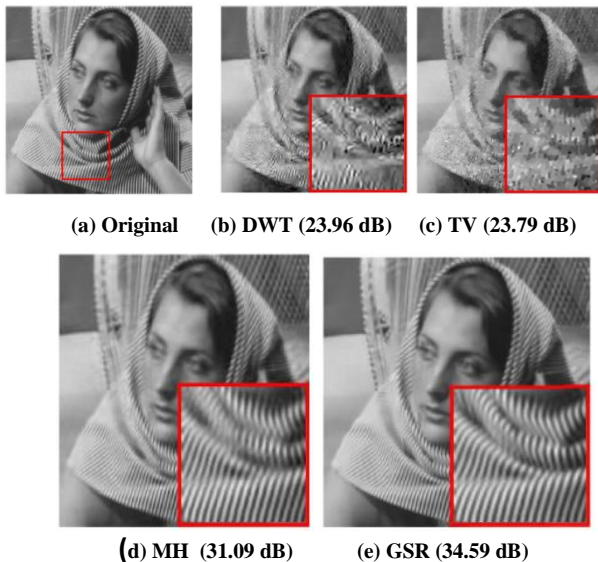
Fig. 2. Results obtained for CS recovery on Barbara with ratio = 20%
