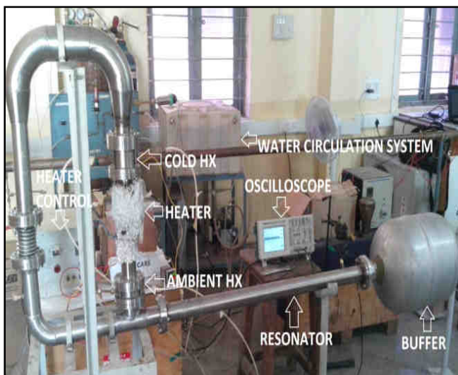
Figure 2 Experimental setup for the TWTAPM
