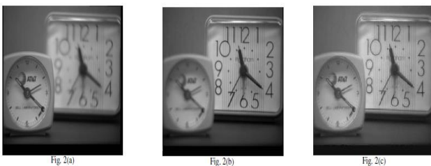
Figure2: (a), (b) original multi-focus image pair (c) Fused image obtained on application of proposed algorithm
