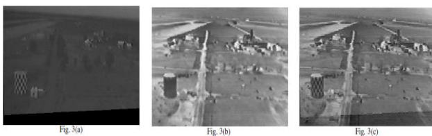
Figure3 : (a) original IR image (b) original Panchromatic image (c) Fused image obtained on application of proposed algorithm
