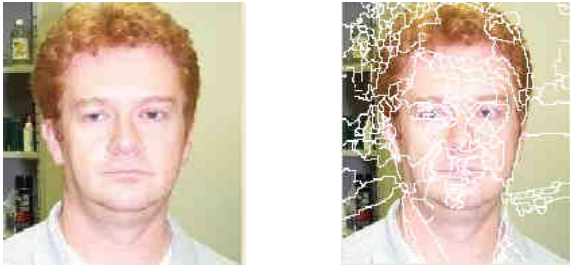
Fig. 2 (a) Original Image (b) Initial Segmented Image by using mean-shift algorithm
