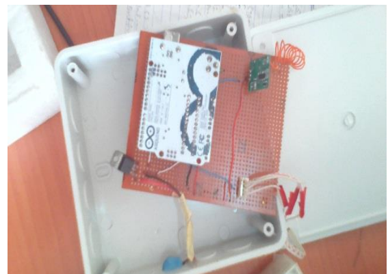
Fig.3.1a: interior view of transmitter unit
