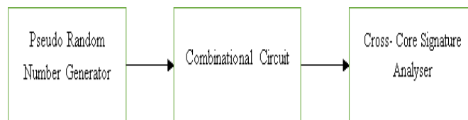
Fig (1) Block Diagram of IC tester
