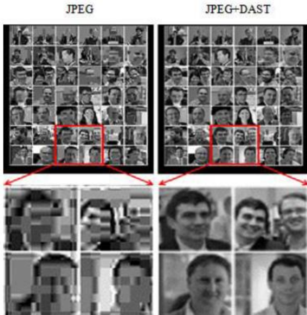
Figure11. Comparison of security and surveillance image using JPEG alone and the case with DAST pre-compression followed by JPEG. In both the cases, DAST +JPEG gives superior performance.
