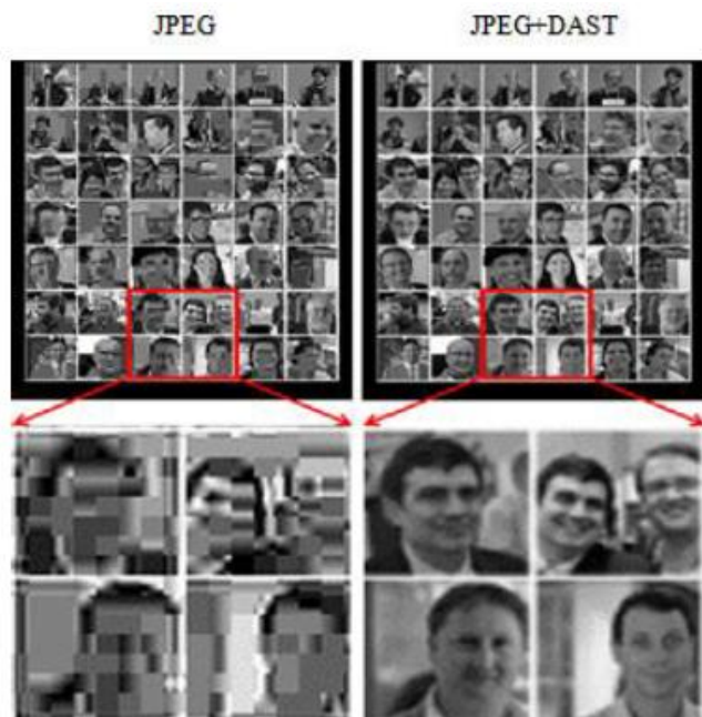
Figure11. Comparison of security and surveillance image using JPEG alone and the case with DAST pre-compression followed by JPEG. In both the cases, DAST +JPEG gives superior performance.
