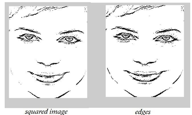
Fig (16) The squared image is a grayscale image transformed to edge binary image
