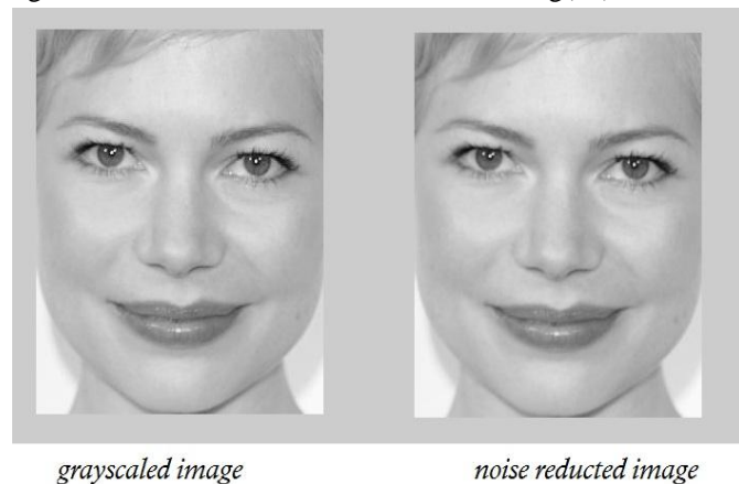
Fig (13) shows the difference in noised and noise reduced image with Gaussian filter
