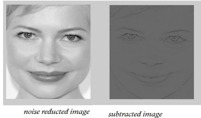
Fig (14) The right image is the result of subtract each adjacent point in a picture.
