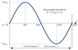
Where: Vmax is the peak value in volts and f is the waveforms frequency in Hertz (Hz).
