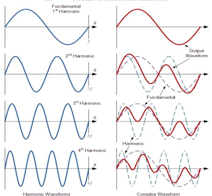
Note that the red waveforms above, are the actual shapes of the waveforms as seen by a load due to the harmonic content being added to the fundamental frequency. The essential waveform can likewise be known as a first harmonics waveform. In this manner, a second harmonics has a frequency twice that of the fundamental, the third harmonics has a frequency three times the fundamental and a fourth harmonics has one four times the key as appeared in the left hand side segment.
