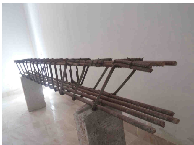
Figure 2: Typical steel cage reinforcement of the beam reinforced with spliced swimmer bars.
