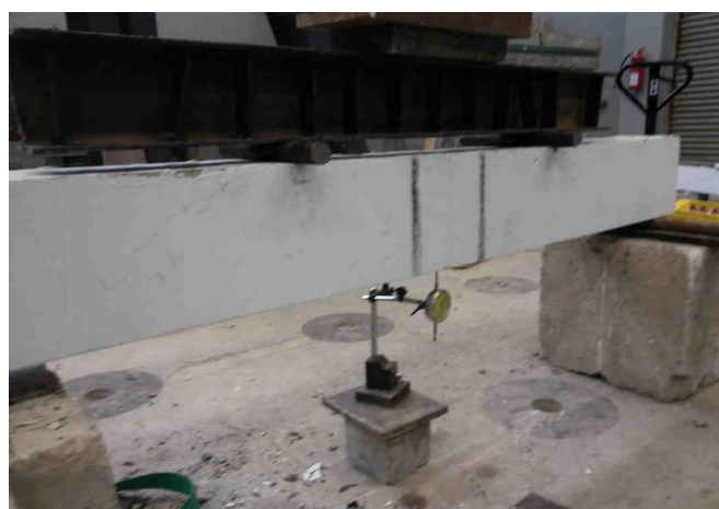
Figure 4: Typical experimental set up and crack monitoring
