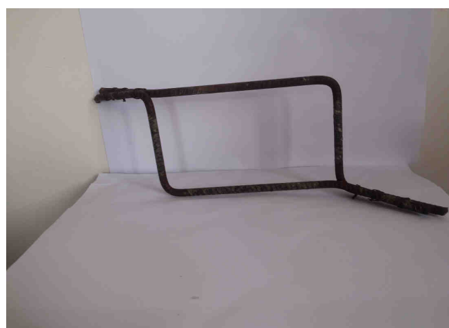
Figure 3: Recycled spliced swimmer bars of new designed shape
