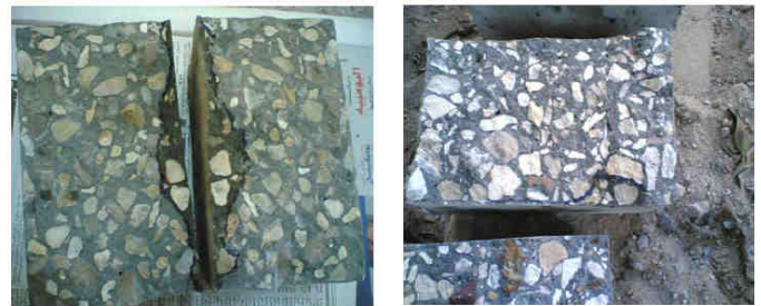
PHOTO (1) DEPTH OF WATER PENETRATION INTO SAMPLE AFTER TEST.
