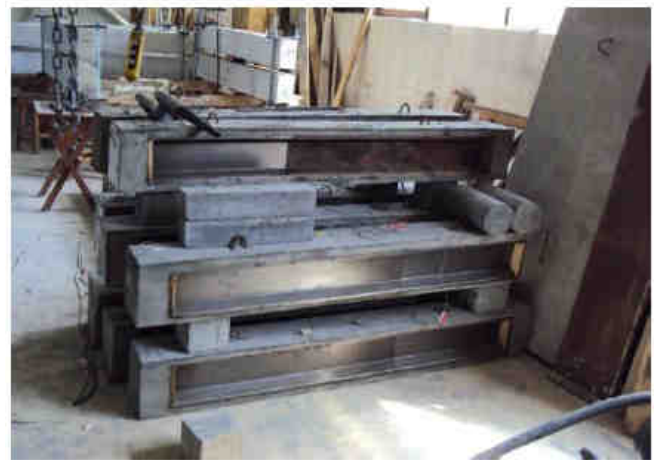
FIGURE (2) REINFORCED CONCRETE SPECIMENS AFTER REMOVING FORMWORK.
