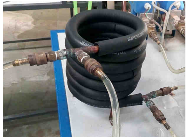
Fig. 3: Actual tube-in-tube helical coil used Specifications of helical coil
