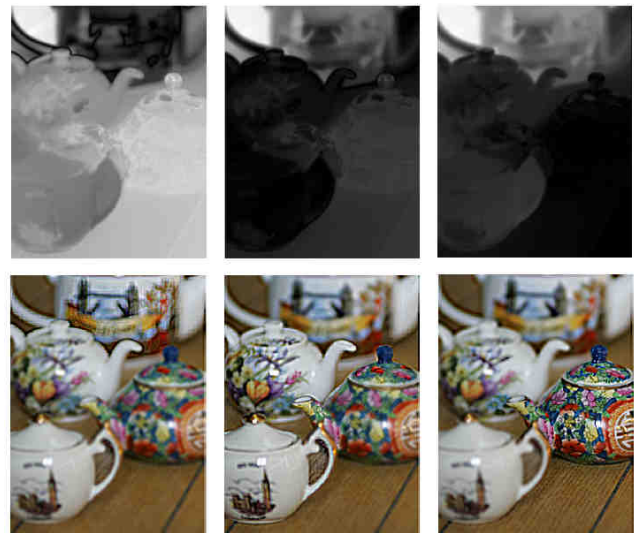
Fig 6. Multifocusing results. Row 1 gives the new blur maps. Row 2 gives the corresponding refocused images.
