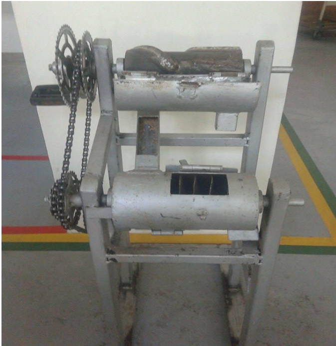
Figure 2 Rice milling machine used in this study
